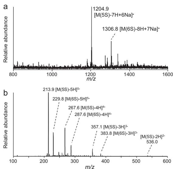
**Fig. 2.** Negative ion IR-MALDI and ESI mass spectra of heparin-derived tetrasaccharide. (a) IR-MALDI reflector TOF mass spectrum. The molecule containing five sulfate groups corresponding to the ion at  $m/z$  1204.9 was present in the sample, but not the fragmentation product. (b) ESI (nanospray) mass spectrum.
