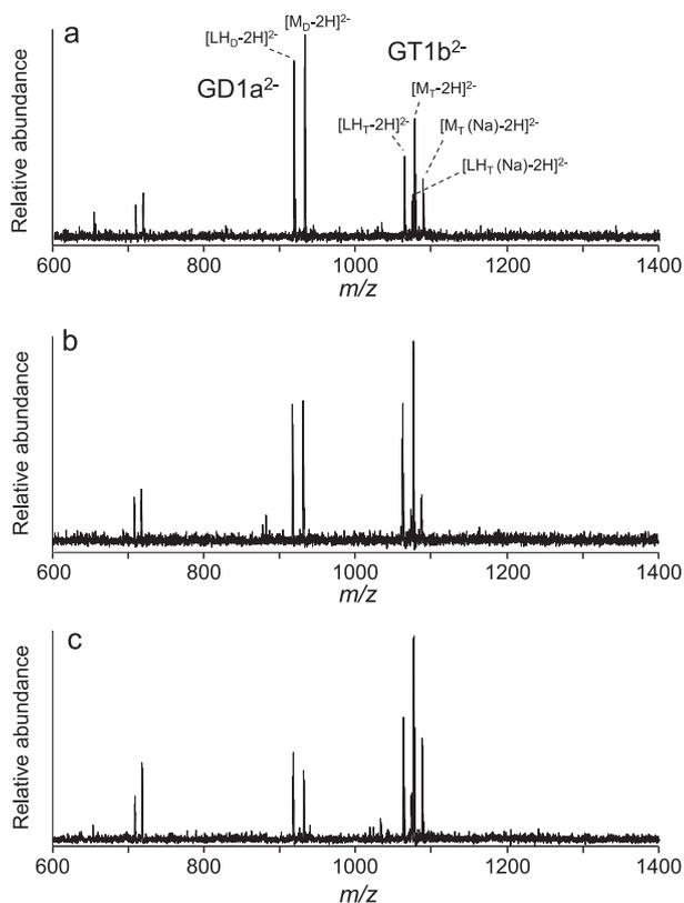
**Fig. 5.** Negative ion IR-MALDI reflector TOF mass spectra of mixtures of GD1a and GT1b gangliosides. The GD1a/GT1b ratios were 2.0 (a), 1.0 (b) and 0.5 (c).
