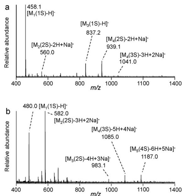
**Fig. 3.** Negative ion IR-MALDI reflector TOF mass spectra of CS oligosaccharides from chondroitinase ABC digestion. (a) Chondroitin (dermatan) sulfate B from pig skin. (b) Chondroitin sulfate E from squid cartilage.
