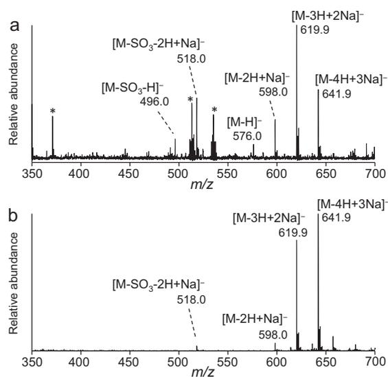
**Fig. 1.** Negative ion MALDI reflector TOF mass spectra of heparin-derived disaccharides containing three sulfates. (a) UV-MALDI mass spectrum with  $\text{G}_3\text{CA}$  ionic liquid matrix. The peaks indicated by an asterisk are matrix-derived ions. (b) IR-MALDI mass spectrum.
