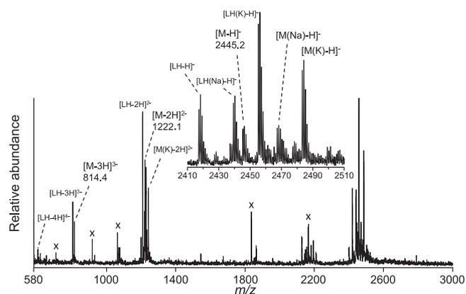
**Fig. 4.** Negative ion IR-MALDI reflector TOF mass spectrum of ganglioside GQ1b. Ceramide structures are C20:1 and C18:1 for M and LH, respectively. The singly charged ion region is depicted in the inset. The peaks indicated by "x" are derived from poorly or desialylated species, which were detected by ESI MS as well (data not shown), and thus were present in the sample before MALDI measurements.
